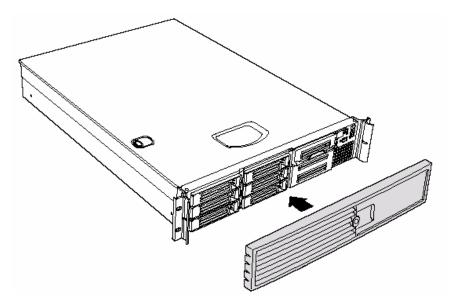
Figure 34: Installing the Front Bezel
